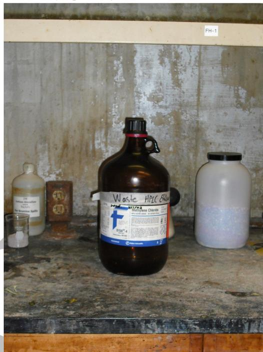
**Figure 3.** Improperly labeled Hazardous Waste container
